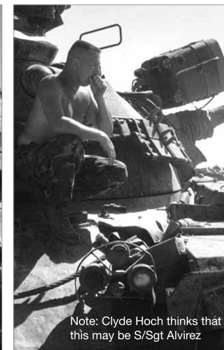
Note: Under the range finder ears and below the track block is an RPG penetration hole.
